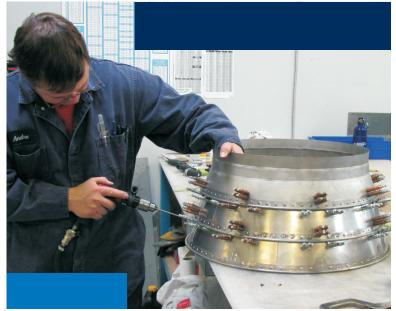
Our aerospace manufacturing experience has been developed through the fabrication of aircraft engine exhaust infrared suppression systems. We have designed and manufactured IR suppressors for the following aircraft types: Bell 212/412; UH-1H; Bell 407; MIL Mi-17; Eurocopter AS332 Super Puma; CASA CN-235; Boeing CH-47; Beechcraft KA350; and the Agusta-Westland AW129. Over 200 aircraft shipsets have been produced at our facility.
